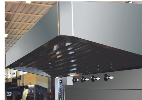
Large AISI 304 stainless steel hood for external/internal aspiration chambers.
